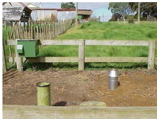
Automatic Telemetered Rainfall Station at Ohaeawai
