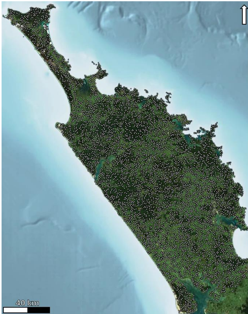
Figure 12 The 7,500 randomly selected sample points across the Northland Region used to evaluate S-PAL alignment with soil and geology classifications.
