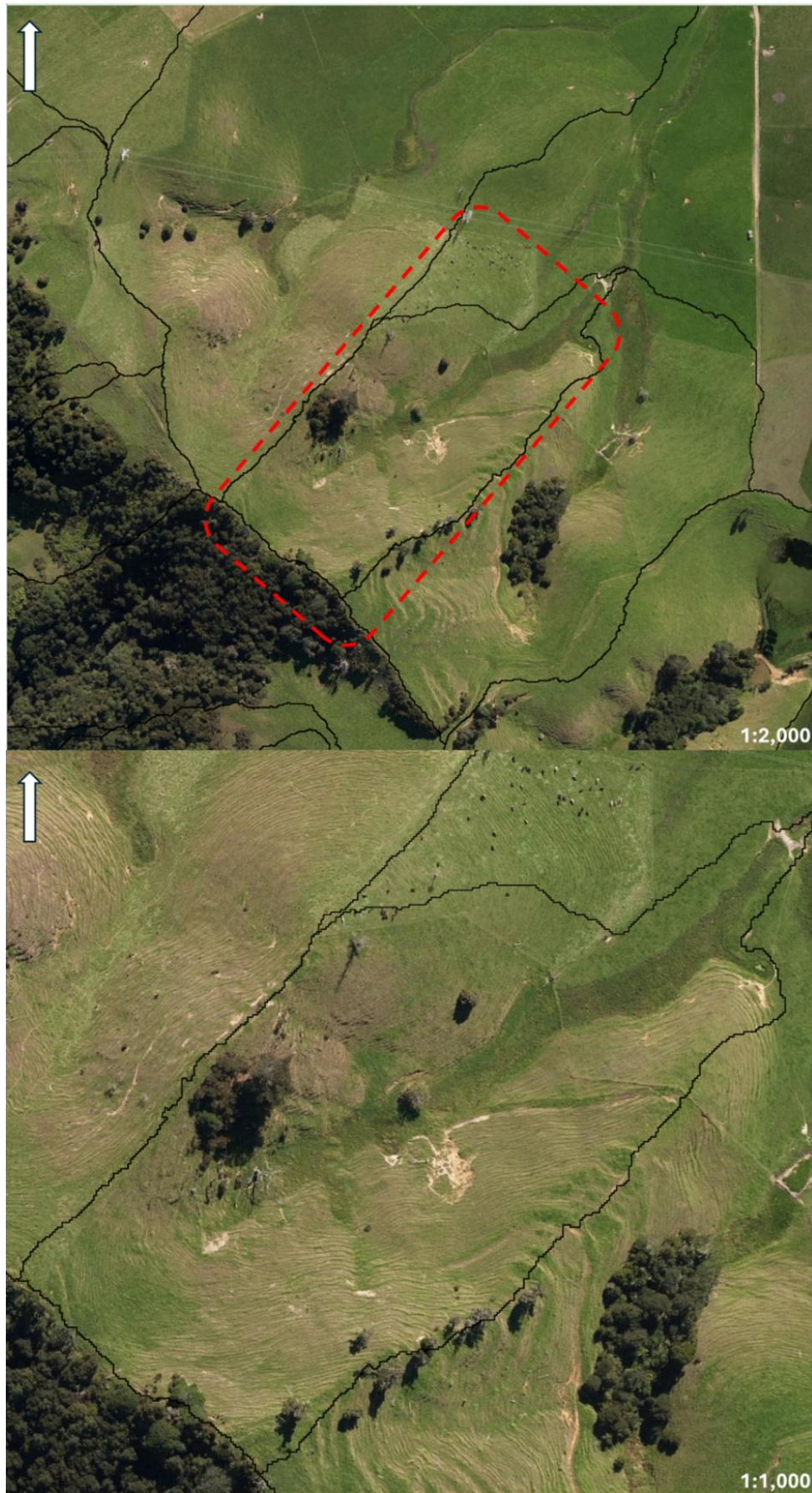
Figure 21. Top: Aerial imagery of extreme soil creep (mass wasting), shallow landslides, and bare soil. Bottom: Zoomed in area within the red dashed rectangle. Visual imagery suggests a high sediment loss potential.
