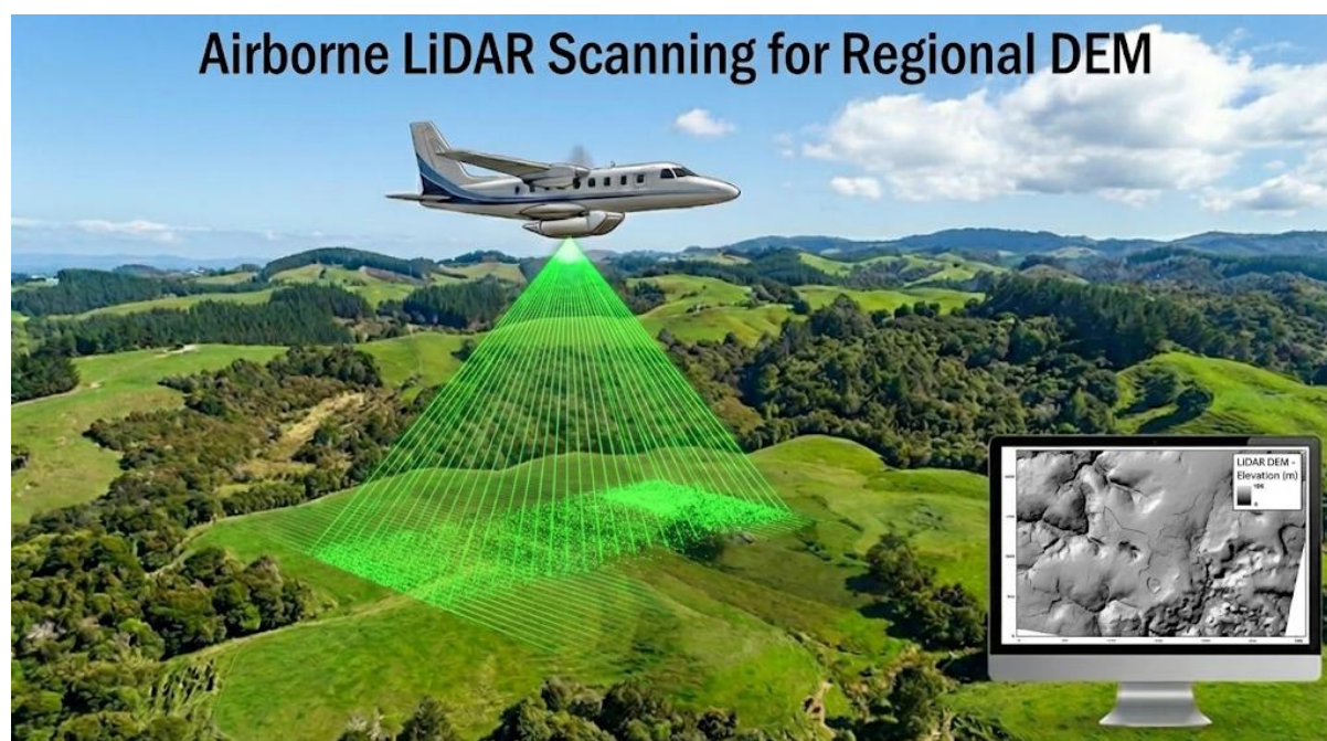
Figure 10. Light Detection and Ranging (LiDAR) survey and inset of Digital Elevation Model. Image LWS.
